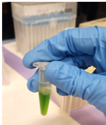
Fig. 4. Liquid-liquid extraction of a plant sample for a lipidomics study. The bright-green layer is enriched in lipid species.
